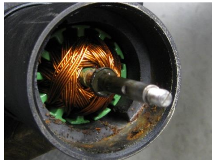
Figure 3 (Water damage to the lower unit)
